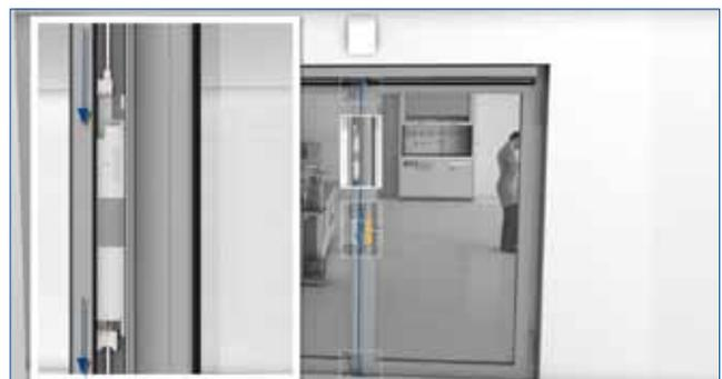
...offers insurance-compliance locking, both in the lintel and in the floor, which reverses the release spring.
