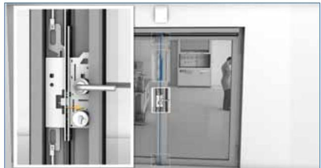
...unlocks the fixed leaf as the motorised unit moves the rod down, simultaneously presses on the strike box, thereby also unlocking the lower rod.
